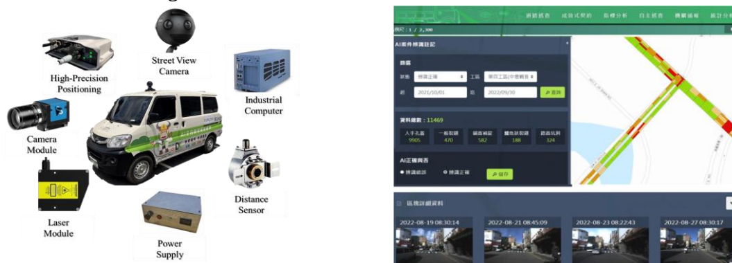
Figure 3 The equipment of the inspection vehicle and the interface of the road maintenance platform.
