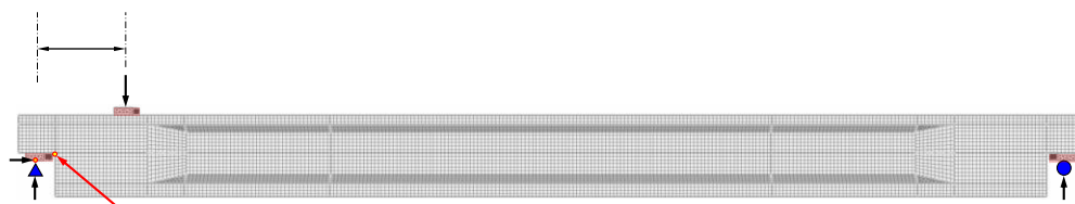
Figure 5 Finite element model of dapped-end girder.
