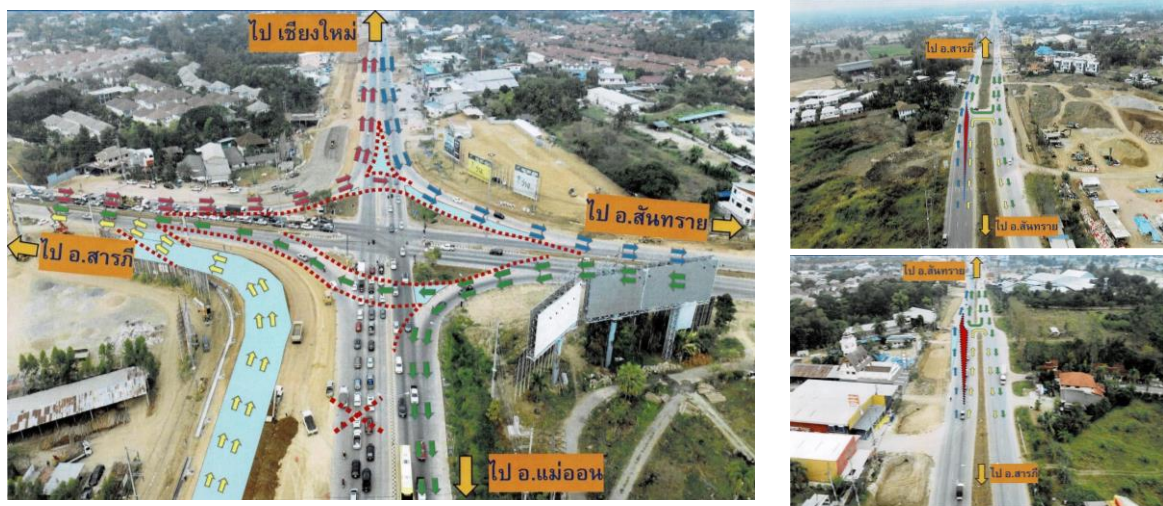
Figure 2 An Example of Median U-Turn Intersection Design for Work Zone Traffic Management (Department of Highways, 2024)
