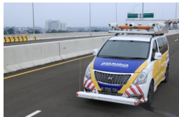
Figure 3 Road survey vehicle Hawkeye 2000. (PT JMTM, 2021)
